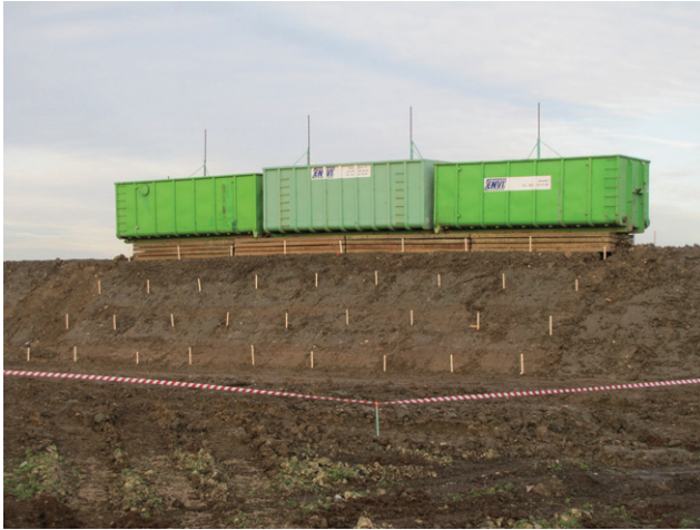
Figure 2. Test set-up of full-scale slope failure test
