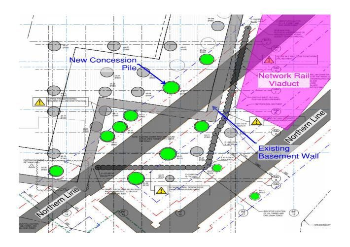
Thanet Sand piles around Northern Line Piles 1m from LUL Concession required ~£70m additional floor space
