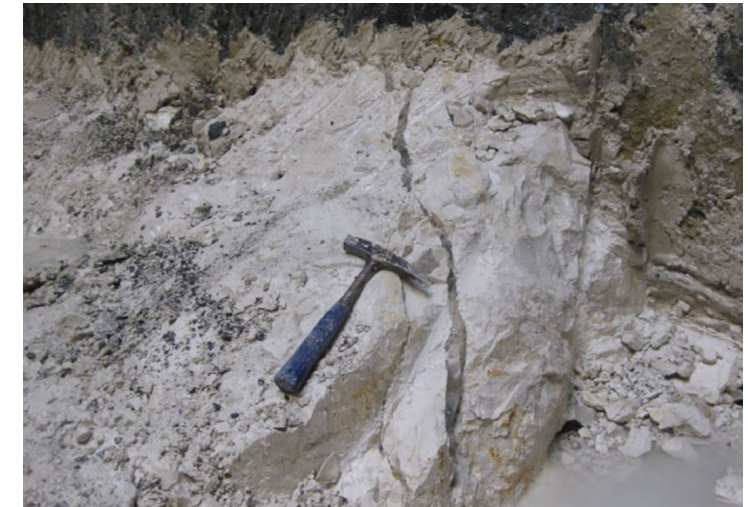
Figure 3 – Identification of grout within fault zone. Confirmed by materials testing
