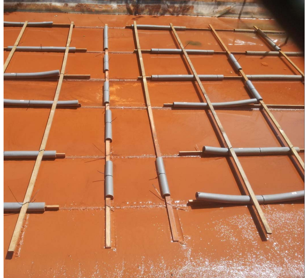
EKG cathodes on top of orches sludge - drying by electroosmosis
