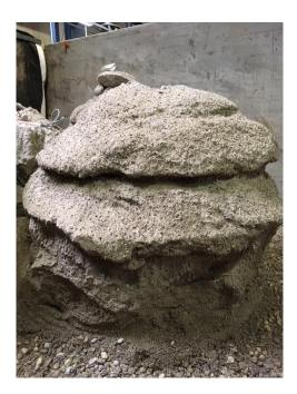
It is based on the injection of ureolytic bacteria with a calcifying solution, which leads to the creation of a biological cement that binds the soil grains together without decreasing the initial permeability. The process has been proven by several experiments, initially on laboratory scale, then in situ on an industrial scale.
